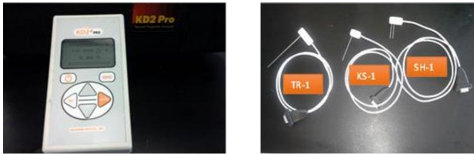
Fig. 4. The measuring device of the thermal features: KD2 Pro
