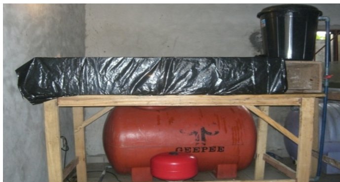
Fig. 1. Solid phase continuous flow biodegradation system
