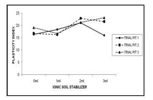
Fig. 6. Plasticity index properties with stabilizer content
