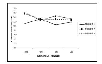
Fig. 7. Linear shrinkage properties with stabilizer content
