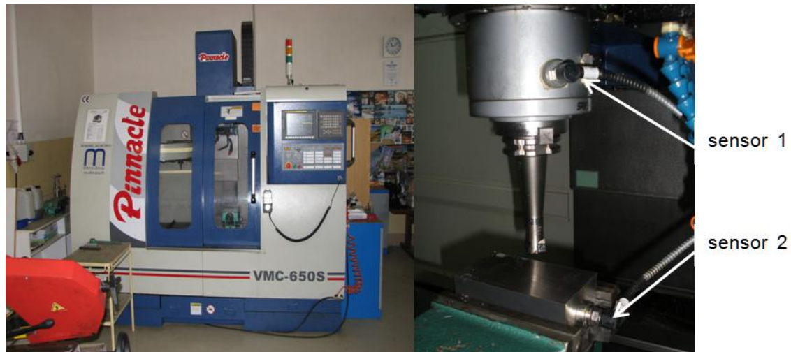
Fig. 3. Vertical machining centre for experiment and detail with sensors
