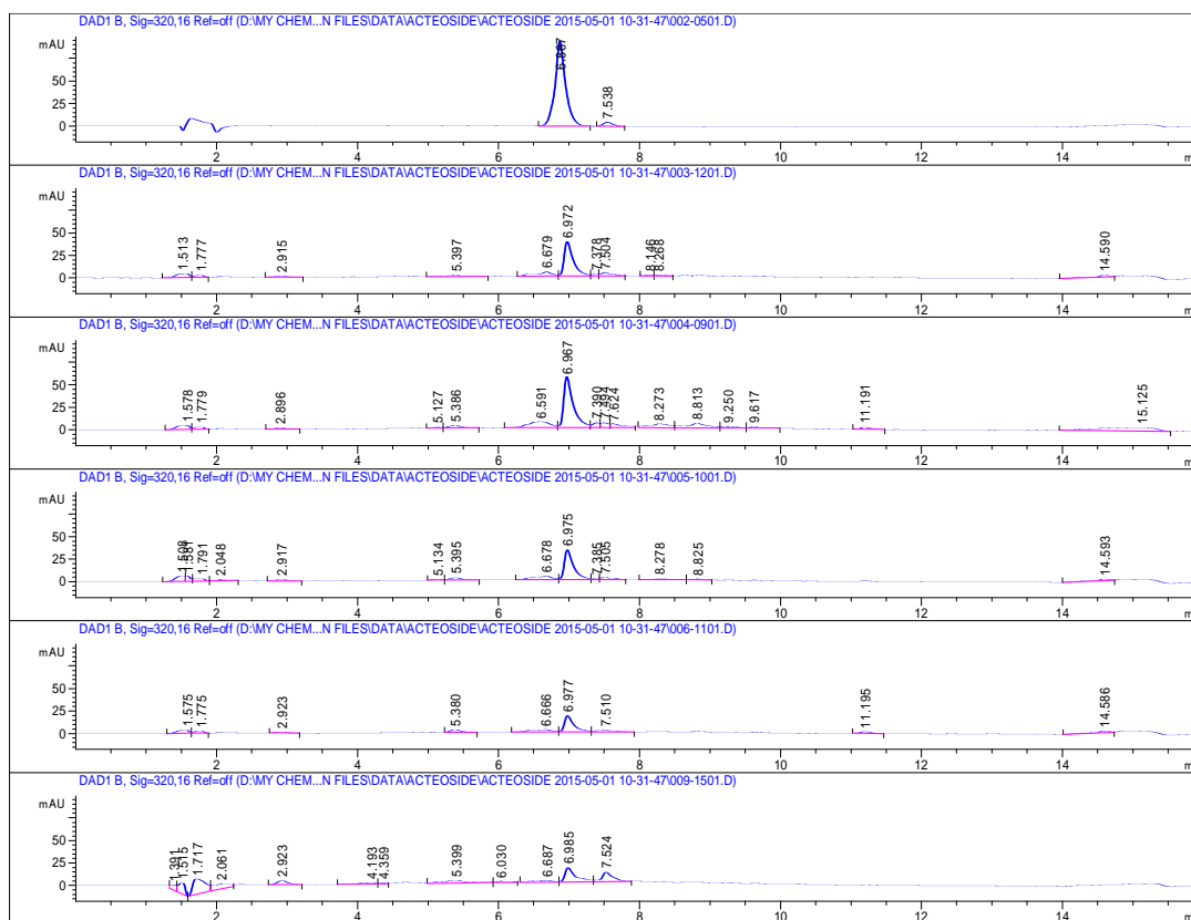
Fig. 2. Superposed HPLC chromatograms of P. lanceolata crude extracts and acteoside standard
