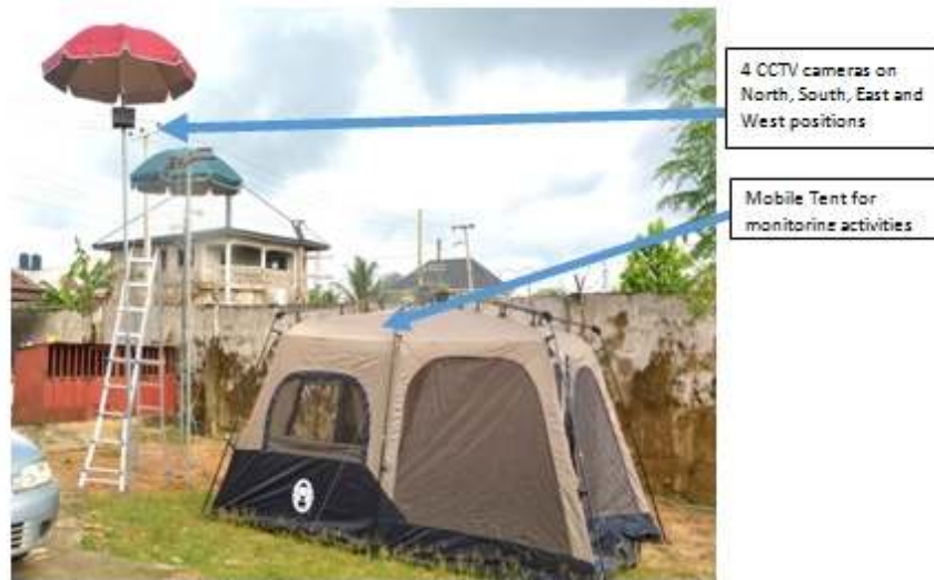
Fig. 4. A typical site set up for the monitoring activities in this study
