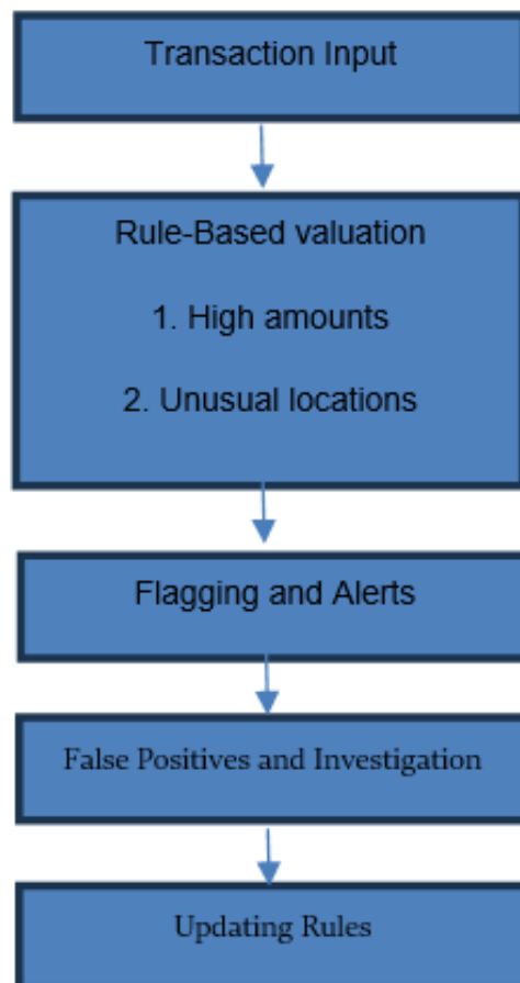
Fig. 5. Representation of Traditional Rule-Based Fraud Detection
