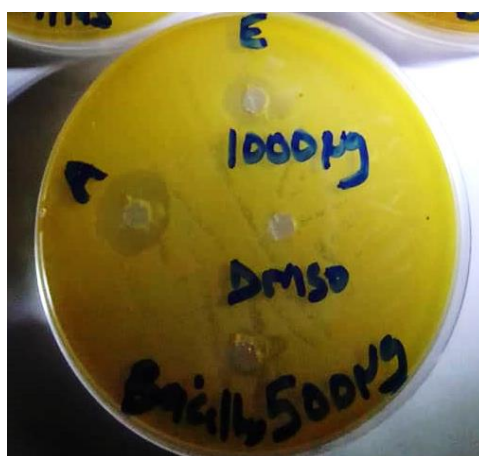
Fig. 9. Bacterial Activities of the ligand(A) and its Cd(II)(B) against B. subtilis by disc diffusion method
