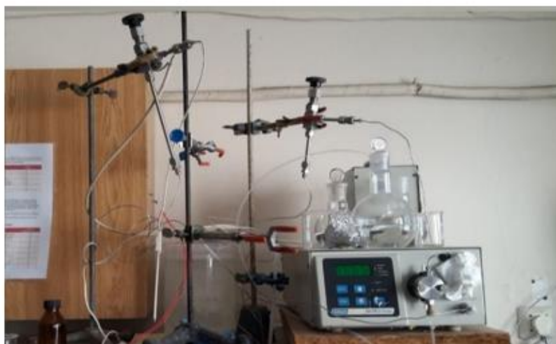
Fig. 5. Superheated water extraction device
