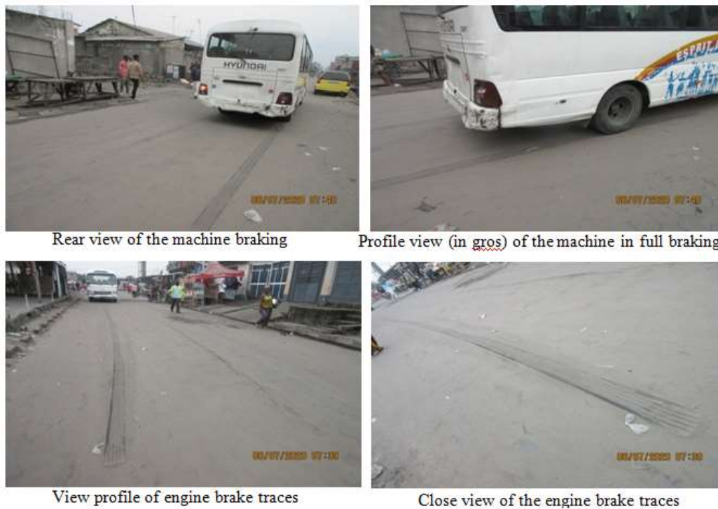
Fig. 6. View of the reaction of the pavers subjected to the adhesion test
