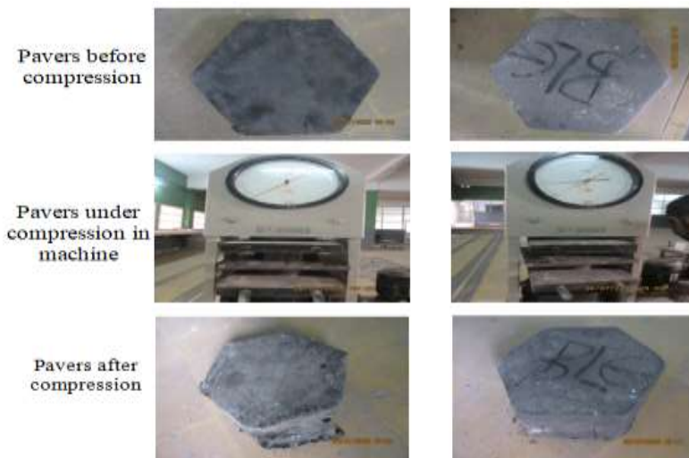
Fig. 3. Reaction of pavers subjected to resistance testing
