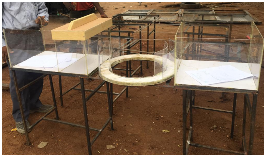
Fig. 2. A set of the U of A mouse anxiety triple test tool (in construction)
