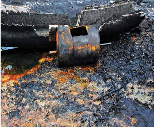
Metal pipes and drums welded together used for boiling crude oil
