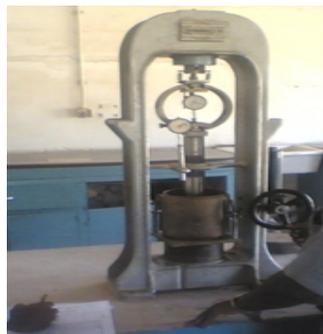
**Fig. 3. CBR test in progress**
