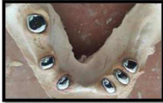
Fig. 5. Metal copings casted from ferritic stainless-steel alloy
