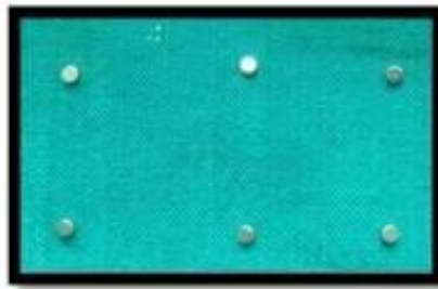
Fig. 10. Nd-Fe-B magnets of dimensions 3x1.5mm
