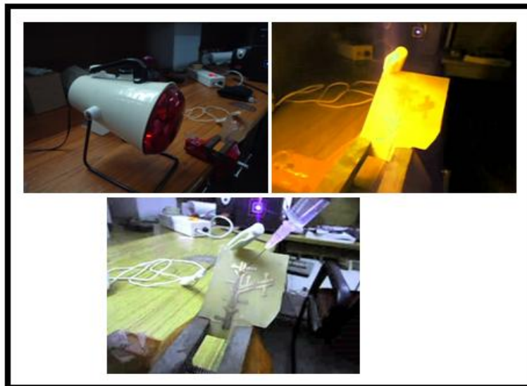
Fig. 2. Temperature control using IR lamp set up
