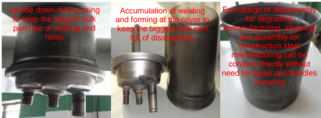
Fig. 6. Eco-design idea to keep the shell bulk with high remanufacturability, using direction is changed upside down to accumulate forming and welding at the cover while and keep bulk free
