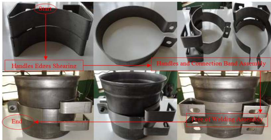
Fig. 10. Remanufacturability due to design for disassembly to certain current power and carbon emission reduction and application of degrading remanufacturing at the end-of-life
