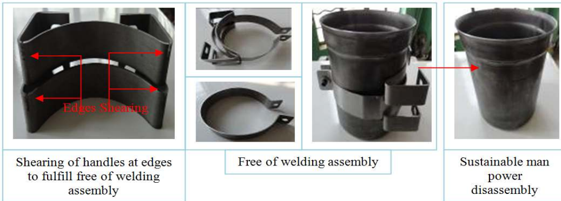
Fig. 9. Remanufacturability due to design for disassembly
