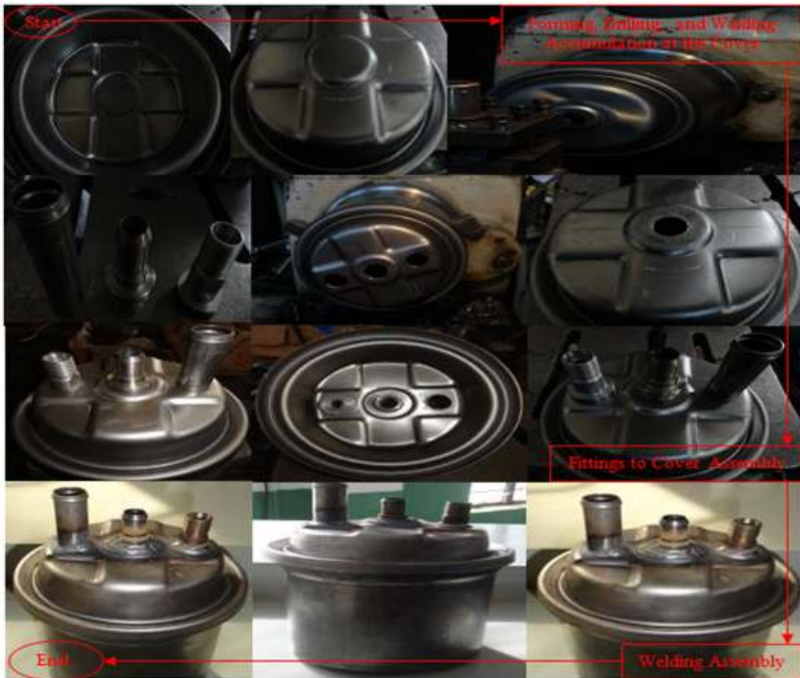
Fig. 7. Eco-design for remanufacturing application for shell hulk free of welding and holes
