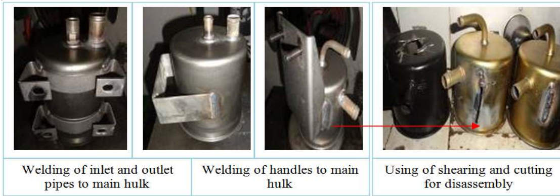
Fig. 8. Non-remanufacturability due to design for non-disassembly by welding
