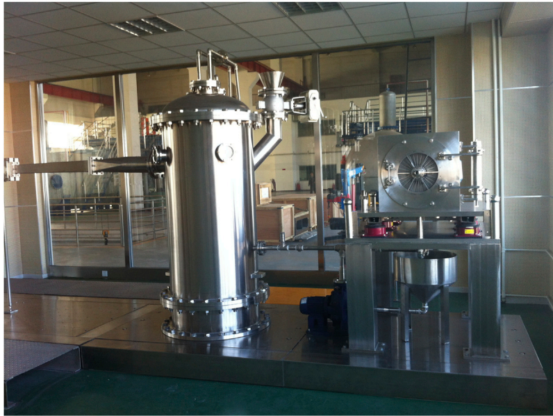
FIGURE 7 Photograph of the hydraulic machinery abrasion testing system at the China Institute of Water Resources and Hydropower Research (Hydraulic Machinery, 2021).
