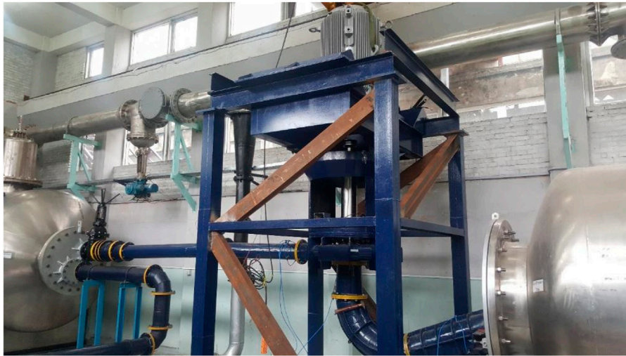
FIGURE 9 Francis turbine test rig under construction at Turbine Testing Laboratory (TTL) at Kathmandu University in Nepal (Thapa, 2019).
