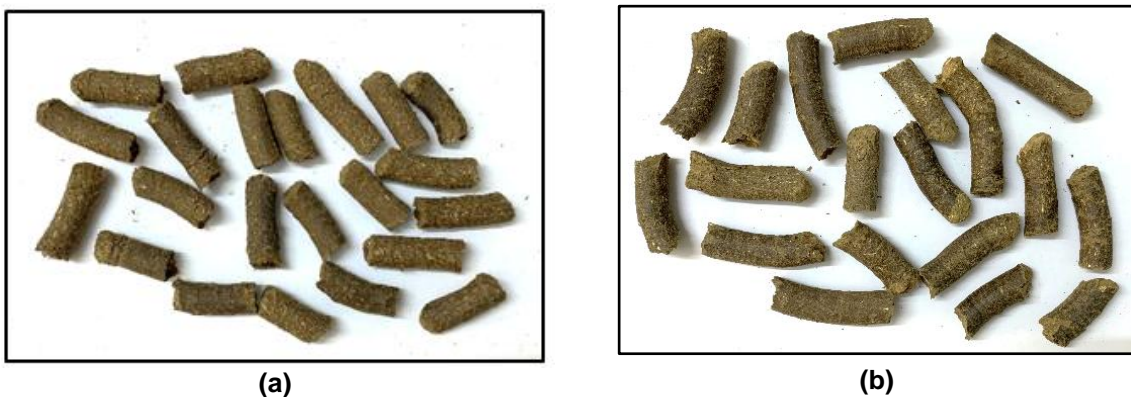
Fig. 2. (a) Soybean straw pellets (b) Cotton stalk pellets produced using flat die type pelleting machine
